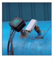
A fully MCERTS approved Electrodynamic<sup>®</sup> instrument replaces non-compliant DC unit on Knockout Sand Plant.
